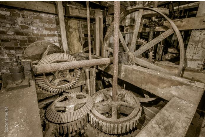
Power for the mill would have originally come from a large wooden wheel in the river outside the building, and was distributed through the building via axles and gears. Cogs on the gears were made alternately of metal and wood, the wood preventing sparks from clashing metal, and reducing the impact of accidental gear jams.
